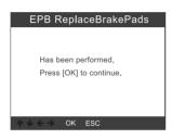
3.1.1 Check whether the brake pump is completely released. The operation of replacing the brake pads is finished, press [ OK ] to complete
