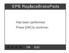
3.2.2. Check whether the retraction is completely, then start to replace the brake pads. After finished, press OK to continue:
