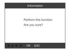
3.3.1. Release Brake Pump, and press [ OK ] to continue:
