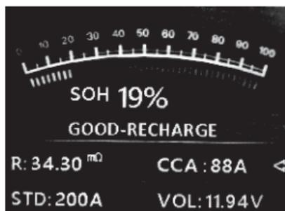
Good battery but low current, recharge before using.
