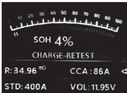
Unstable battery shall be recharged and retested to avoid error. If the same test result appears after recharge and retest, the battery is regarded as damaged, replace the battery.
