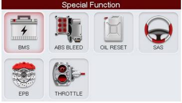
Press [BMS], the screen displays the areas and vehicle for BMW starting.
