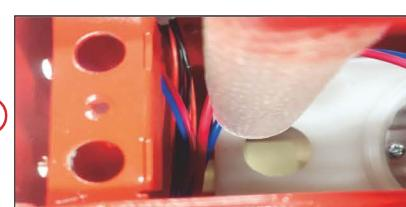
Align the hose with the hole in the tank.
