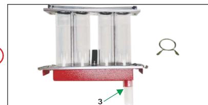
Insert the hose(3) into the drain port.
