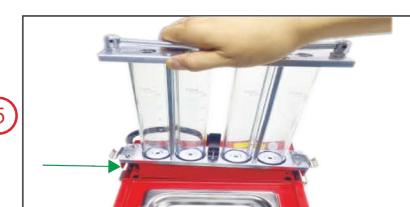
Take the glass assembly above the mounting hole of the main unit, and the fuel hose is on the left.
