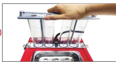
⇒ Press down the glass assembly to keep both sides installed horizontally.
