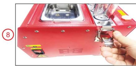
Hang the hook of the fixing mechanism on the assembly.
