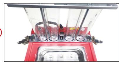
The hook on the fixture is hung with the glass assembly.
