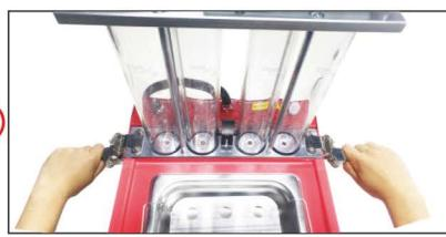
⇒ Press down on the fixings on both sides.
